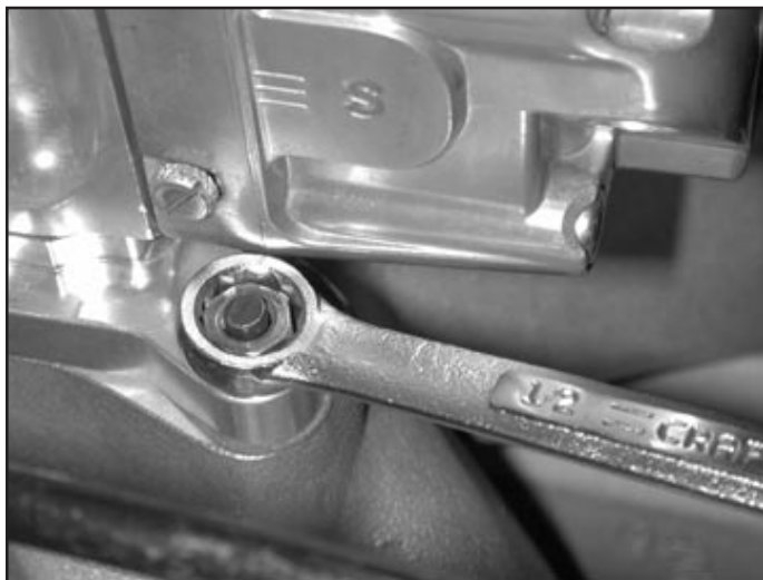
A socket or standard open-end wrench must be used to tighten the carburetor to the manifold.
