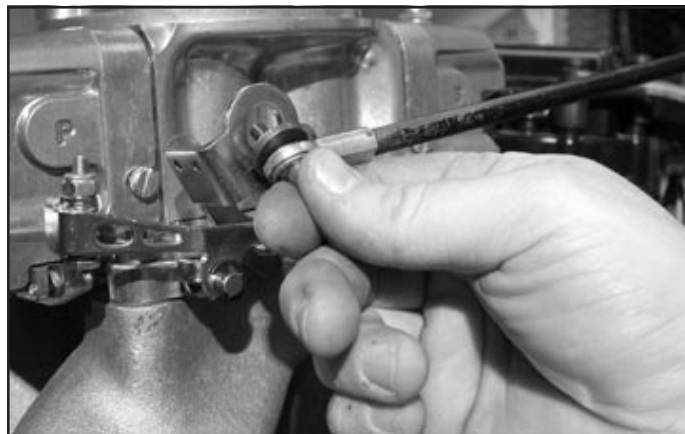
Install the throttle linkage to the throttle arm using a carburetor throttle link bushing (part #160009)
